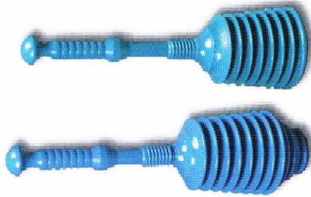
The bellows-style plunger for a toilet (left) has a narrowing plunging end to fit inside the bowl and create a better seal; those designed for flat drains (right) have a flat bottom to better seal a drain in a sink, tub, or basin.
